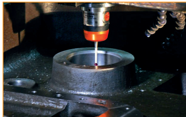
The Primo Radio Part Setter inspecting the turbocharger housing
